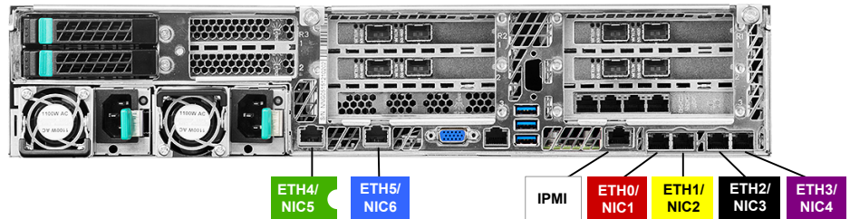
Figure 1-9 NetBackup 5240 Appliance rear port color codes
